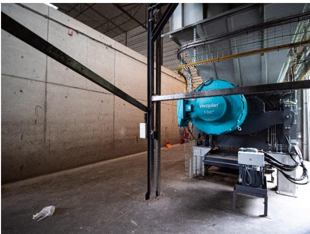
Photo 2: The HiTorc drive is very efficient and is insensitive to impurities. In comparison with belt and hydraulic drives, it requires hardly any maintenance.
