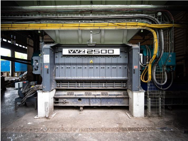
Photo 1: Vecoplan installed a VVZ 2500 T shredder. This double-shaft shredder efficiently processes even difficult and contaminated materials such as domestic waste.
