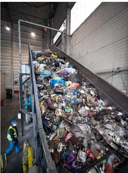
Photo 4: FBSerwis can process 42 tonnes of material per hour with the new Vecoplan system.
