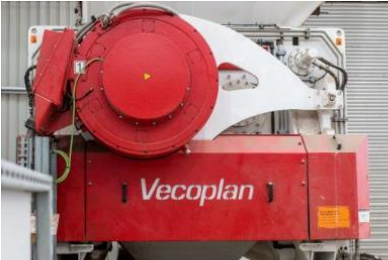
Photo 3: The heart of the system is a VNZ 2500 XL-T double-shaft re-shredder from Vecoplan.
