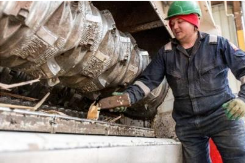
Photo 1: Vecoplan's shredder is equipped with a flipper system that prevents damage to the machines from impurities and simplifies removal of foreign objects.
